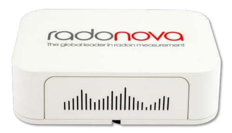
The OY1500 LoRaWAN Radon gas sensor is designed to measure radon gas, temperature, humidity and pressure. It also has an accelerometer to detect movement of the device. The device is designed to operate indoors powered by cable or with a battery life length of 60 days, with rechargeable batteries. It reports every 10 minutes, allowing for quick adjustments of ventilation systems when radon levels get too high.
