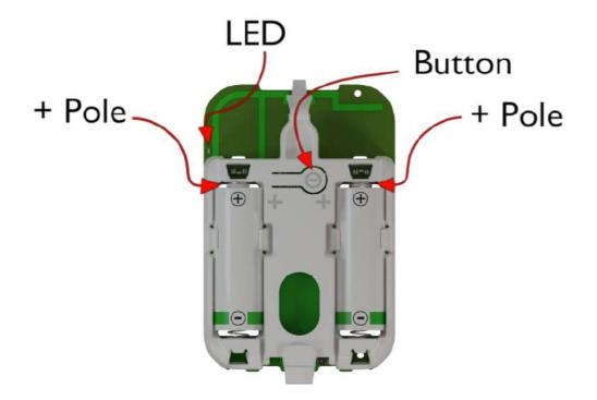
Configure the device in the LoRaWAN server, according to chapter 6.1, and insert the batteries. The sensor starts and flashes 2 + 6 times during the boot-up sequence. The sensor is activated by pressing the push button for 3 seconds until the red LED makes two short flashes. When the device has successfully joined the LoRaWAN network there will be a 2-second-long flash. Attach the electronic board to the bottom piece and attach the plastic cover.
