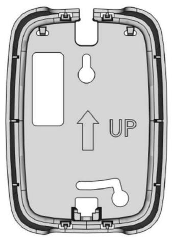
The bottom piece is mounted on the wall with the "UP" arrow upwards. It can be mounted either with screws or adhesive tape.
